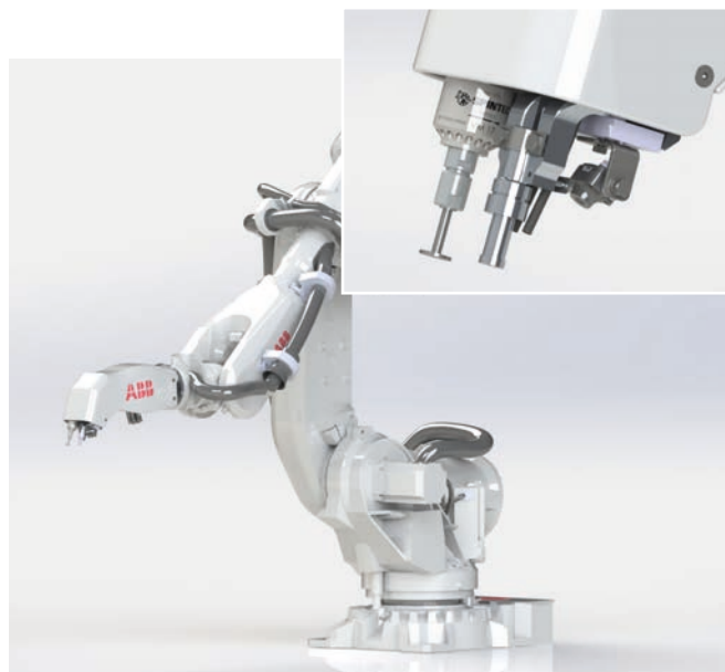
Fig. Example of an integration: ABB robot with PHAsisBLU ultrasonic device and probe, incl. coupling agent spray unit and surface milling cutter
